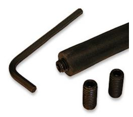
Commercial threaded end-plugs. These devices are threaded like the bolts mentioned above, but use an Allen drive to thread them in. They are made of anodized steel. They do not have the big head of the hex-head bolt, so present less of a hazard should they come loose on the roadway. You must specify what size center hole you will be plugging. These are of moderate cost.
