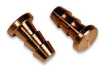
Commercial brass end-plugs. These devices are barbed and just press into the end of the hose. You have to specify what size center hole they are designed for. These can be purchased with a pin-hole for hot temperature use. These are high cost, more so when a pin-hole is needed.
